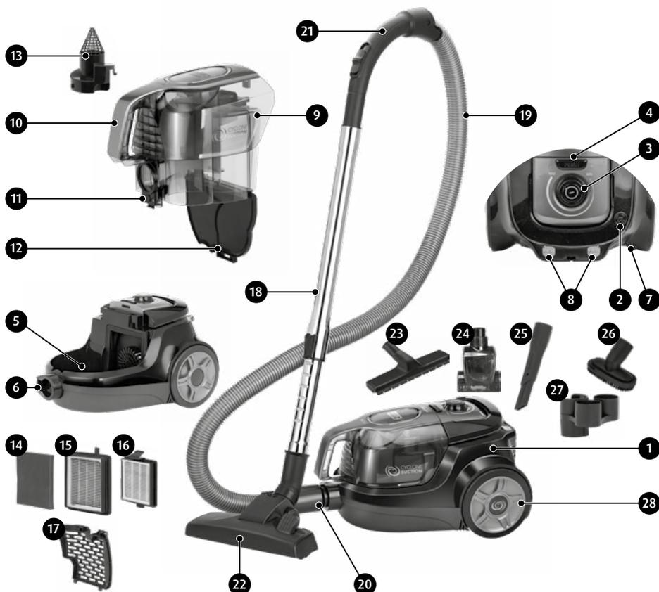
Unlike traditional vacuum cleaners, this bagless cyclone vacuum cleaner feature no bag for collecting dust and debris. Instead, the appliance has a purpose-designed cyclone chamber, in which air is forced to rotate in a vortex at an extreme speed. This creates a centrifugal force which expels all dust and debris collected by the vacuum cleaner to a dust canister. The dust canister is cleaned with ease. Using the cyclone vacuum cleaner saves time and reduces operating costs of the appliance
