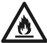
caution, risk of fire
